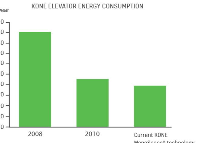
The calculation is based on an elevator speed of 1 m/s, a load of 1600 kg, 200,000 starts/year, a travel height of 16 m and 5 floors
